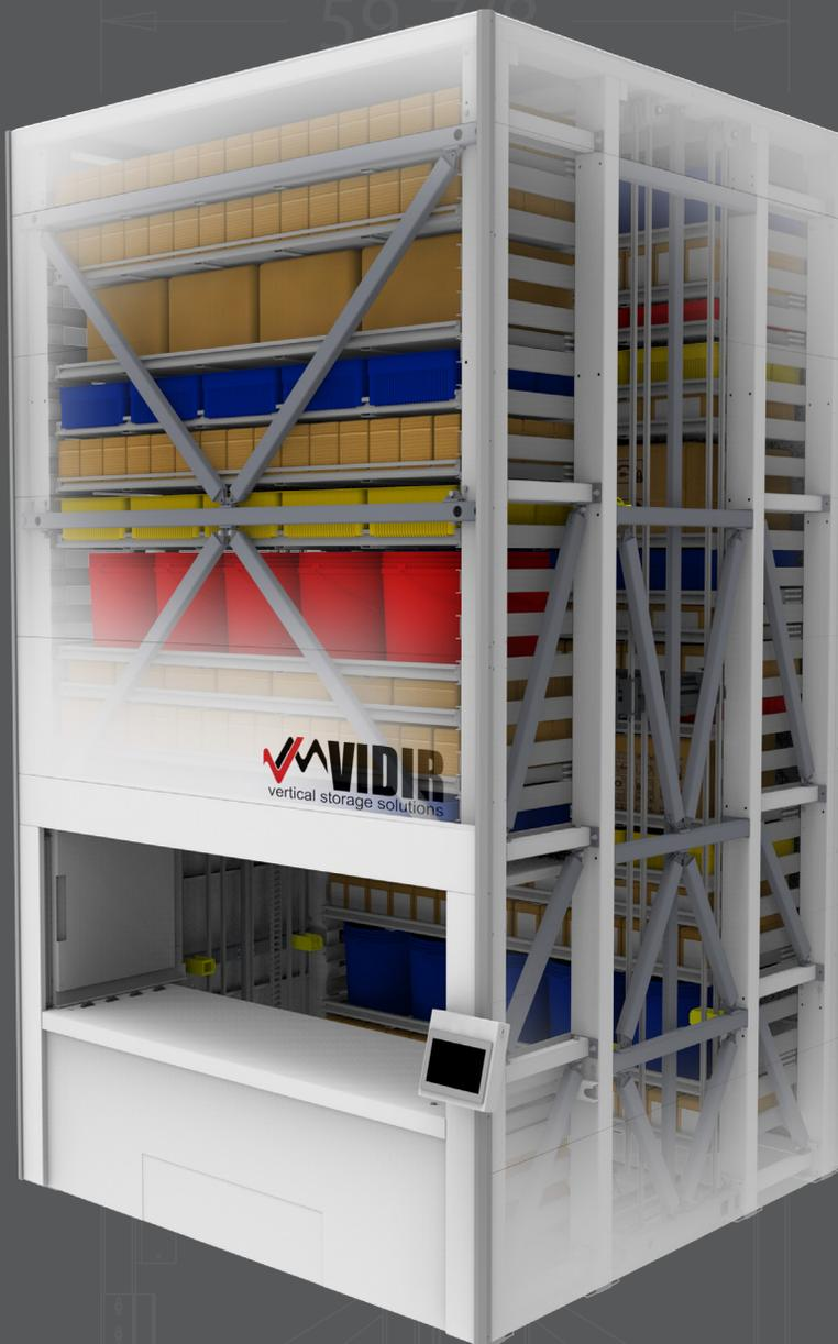
The Vidir Lift Module (or VLM) is Vidir's revolutionary new automated storage and retrieval system that provides smart, adaptable storage to maximize density and further increase productivity. Making use of 2 tray towers, one in front and one in back, along with a center elevator, trays are extracted and presented quickly, efficiently, and at an ergonomic height. Storing the trays in vertical towers allows for a minimal footprint, saving floor space up to 85%.
