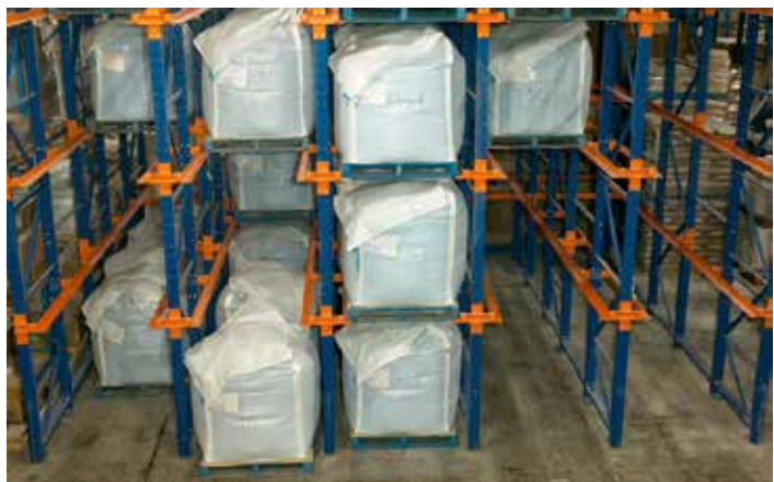
Drive-in/Drive-thru rack for multiple pallets of same products
