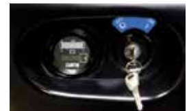
Battery discharge indicator and key switch.
