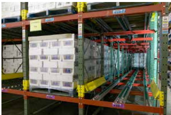
Pallet Flow for products requiring first-in first-out storage
