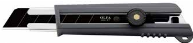
Model # NH-1 -Premium Ergonomic Rubber Grip " Hand Saver" Handle - Ratchett Lock - Elastomer resin handle is chemically resistant to paint, paint thinner and MRO environments.
