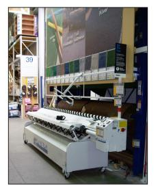
**Cut n'Roll** Power Cutter and Roll-up system, state of the art electronic counter, belted roll-up cradle, simple one-person operation
