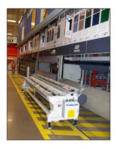
Rack n' Roll Power cutter and roll-up system, rotary cutter design, simple one-person operation
