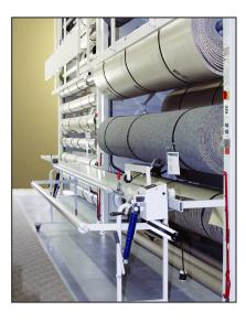
Carousel Mate Manual cutter and roll-up system, built-in measuring system
