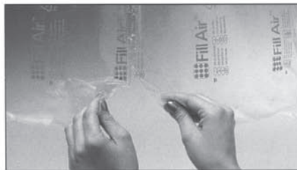
Step 2: Once the desired cushion size is selected, tear off as many inflated cushions as needed.
