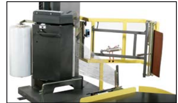
Orion Insta-Thread™ film carriage and film tail treatment mechanism on Flex LPA (top) and Flex HPA (bottom).
