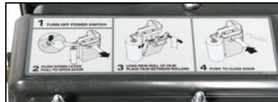
Graphic instructions on top of the carriage guide the operator through film threading.
